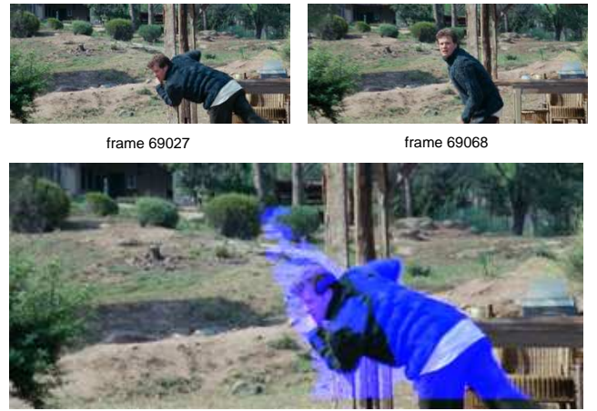
Figure 7: Motion detection: the actor is moving both before and after the cuts, so the motion is detected, and what started as a large area of discrepancies is instead given a consistent explanation as motion in the scene (and coloured blue to indicate this). Because of the unusual pose of the actor in these images, the upper-body-detector could not be expected to identify this as a human.
